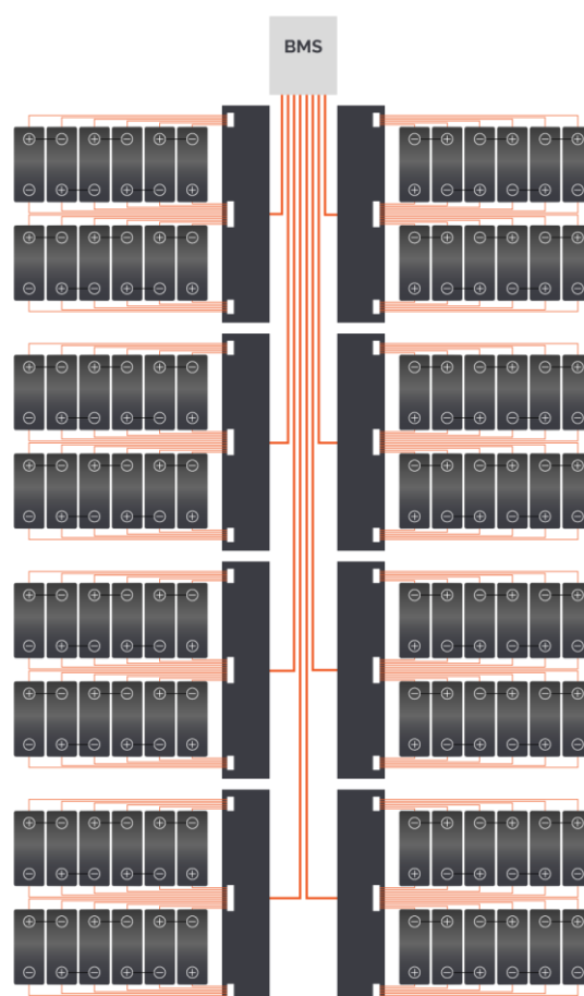
Figure 1: A traditional wired battery design with modularized cell grouping
