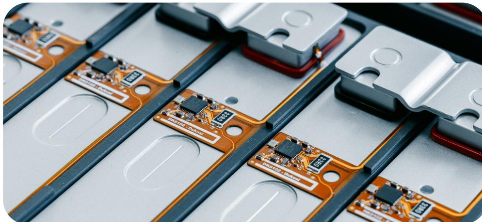
The Dukosi Cell Monitoring System (DKCMS) consists of DK8102 Cell Monitors, a DK8202 System Hub, and the Dukosi API. The Cell Monitors make accurate, synchronous, on-cell measurements, process the data, and send it to the BMS main processor (Host) via the System Hub. Dukosi's proprietary C-SynQ<sup>®</sup> communication protocol provides bidirectional communication between the System Hub and the Cell Monitor network, which is managed by the System Hub and Dukosi's API.
