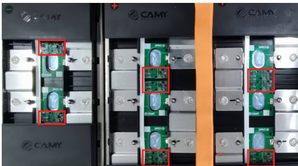
Each cell is affixed with a Dukosi Cell Monitor (highlighted red) that accurately measures cell voltage and skin temperature. All cell data is captured synchronously and transmitted with deterministic latency via C-SynQ communication via Dukosi System Hub to the BMS host processor.
