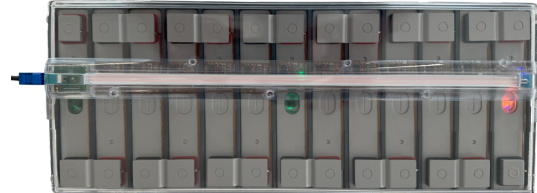
After the lid is closed on the enclosure the integrated antenna overlays the row of near field antennas from each Cell Monitor.
