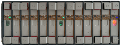
Prismatic cells with Dukosi's Cell Monitors installed on each cell
